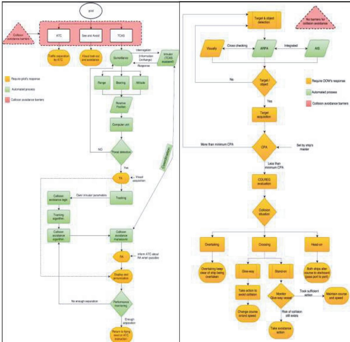
**Fig. 3.** Collision avoidance procedures in aviation      **Fig. 4.** Maritime collision avoidance procedures
