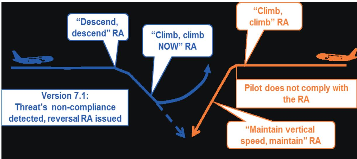
Fig. 2. TCAS RA to avoid collision (EUROCONTROL, 2016)
