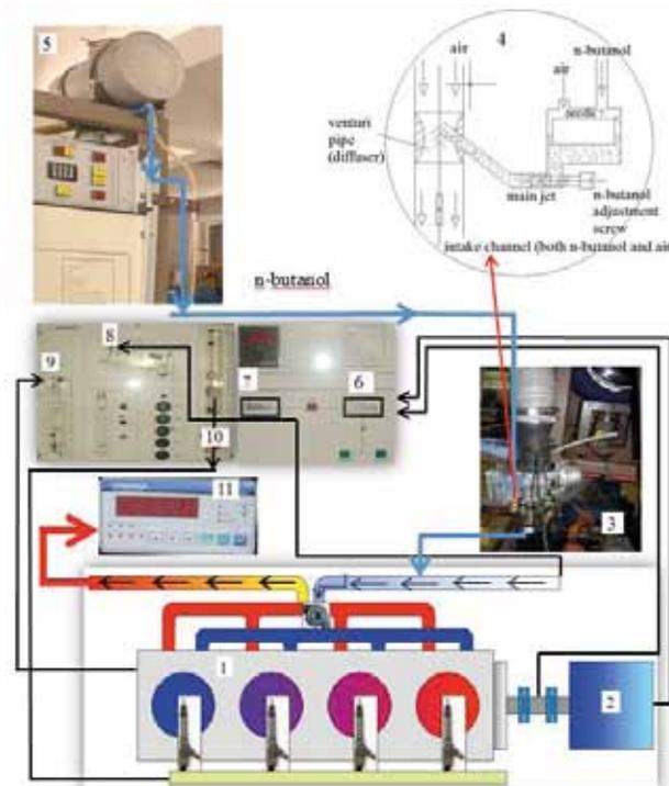
**Figure 1.** Experimental system. 1-engine, 2-loading unit, 3- adapted carburetor, 4- technical drawing of the adapted carburetor, 5- n-butanol tank, 6-force, 7-speed, 8-air measurement manometer, 9- coolant flow meter, 10-fuel measurement unit, 11- gas analyzer (NO<sub>x</sub> analyzer).
