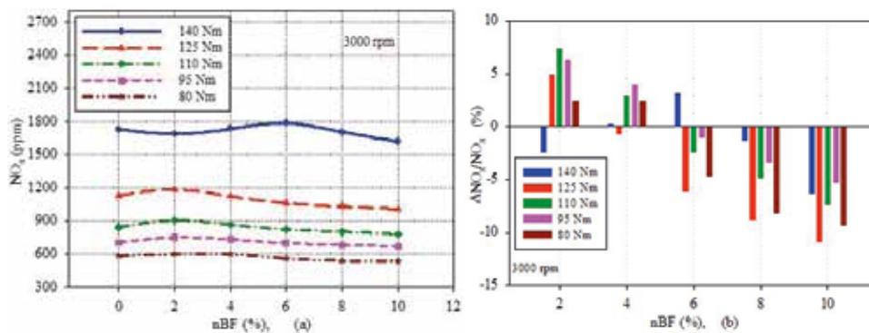
**Figure 8 (a and b).** Variations and variation ratios of NO<sub>x</sub> versus different n-butanol ratios under five different loads, respectively.
