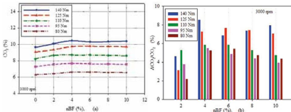
**Figure 6 (a and b).** Variations and variation ratios of CO<sub>2</sub> versus different n-butanol ratios under five different loads, respectively.
