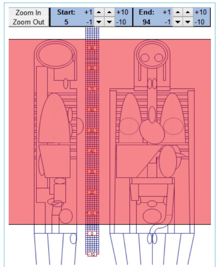
**Figure 1.** Mathematical phantom used with imPACT software to compute patient doses covering the head, chest and abdominal-pelvic region.
