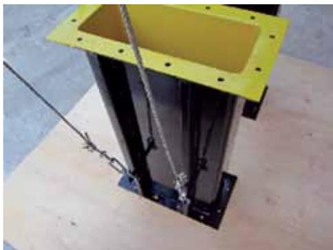
**Figure.9** Distance unit with steel wire rope.
