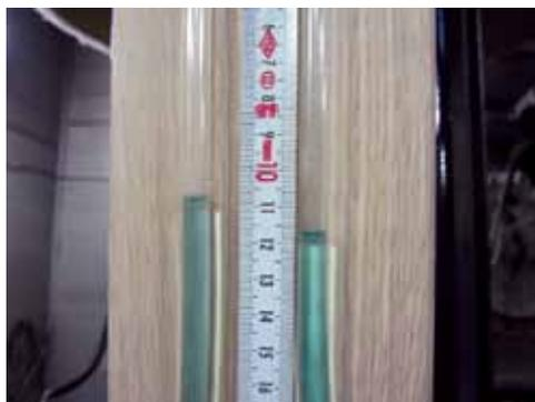
**Figure.11** Visual pressure drop measurement, U-manometer.
